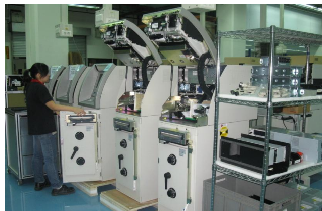
Figure: A factory is manufacturing ATMs. Vaults and dispensing units are seen in the picture.
